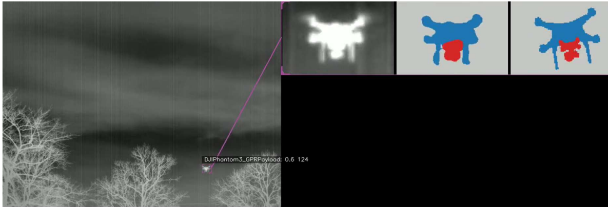
Figure 6: ZEUS pipeline evaluated on FLIR BOSON IR sensor data at an internal demo. In this footage, a DJI Phantom 3 carrying a Go Pro payload is correctly classified by our pipeline.
