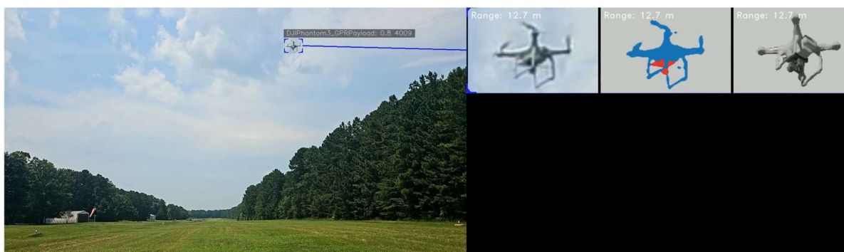
Figure 5: ZEUS pipeline evaluated on BASLER EO sensor data at an internal data collect. The left image corresponds to the full detection input frame. The row of chips to the right correspond to outputs of the pipeline. From left-to-right, the UAS image chip is recovered by the detector, receives a drone-payload pixel mask by our segmenter, which is then assigned to a model library match. For visualization purposes, a 3D render of the matched CAD model is shown at its predicted pose. At the top left of each image chip, the result of the passive ranging module is shown in meters.
